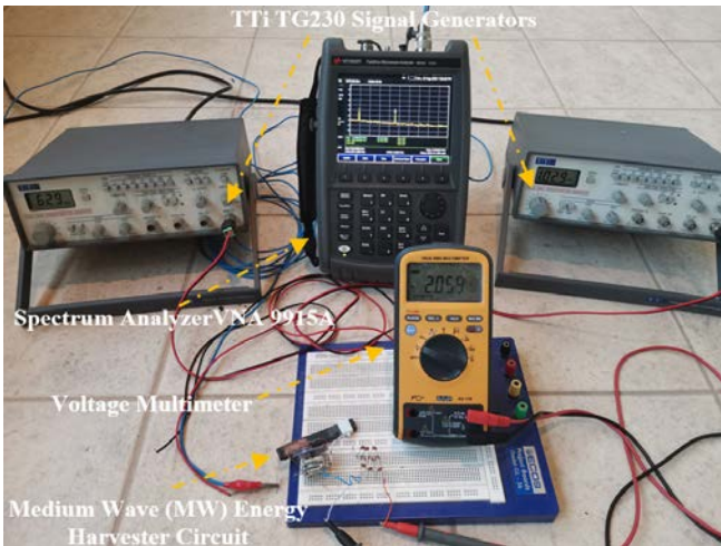
Fig 6. The experimental setup by the utilization of TTI TG230 laboratory signal generators with Amplitude Modulation ( Full-AM ) features.
