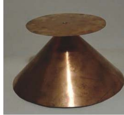
Fig. 2. Discone antenna prototype from copper foil, with inner cone angle 90^\circ , height 12 cm and low-cut frequency 750 MHz
