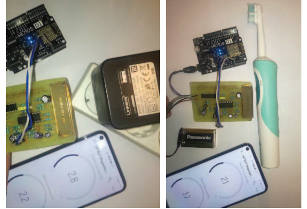
Fig. 5. Measuring the magnetic flux density of various devices by the proposed IoT-based meter. The ELF field strength values ( in A/m and Tesla ) are displayed on the Blynk application supported by the Android platform in a mobile phone with Wi-Fi network connectivity as a complete IoT solution.
