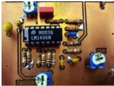
Photo 2. The modulator is based on the well known MC1496 IC, which is able to suppress the carrier for more than 60db
